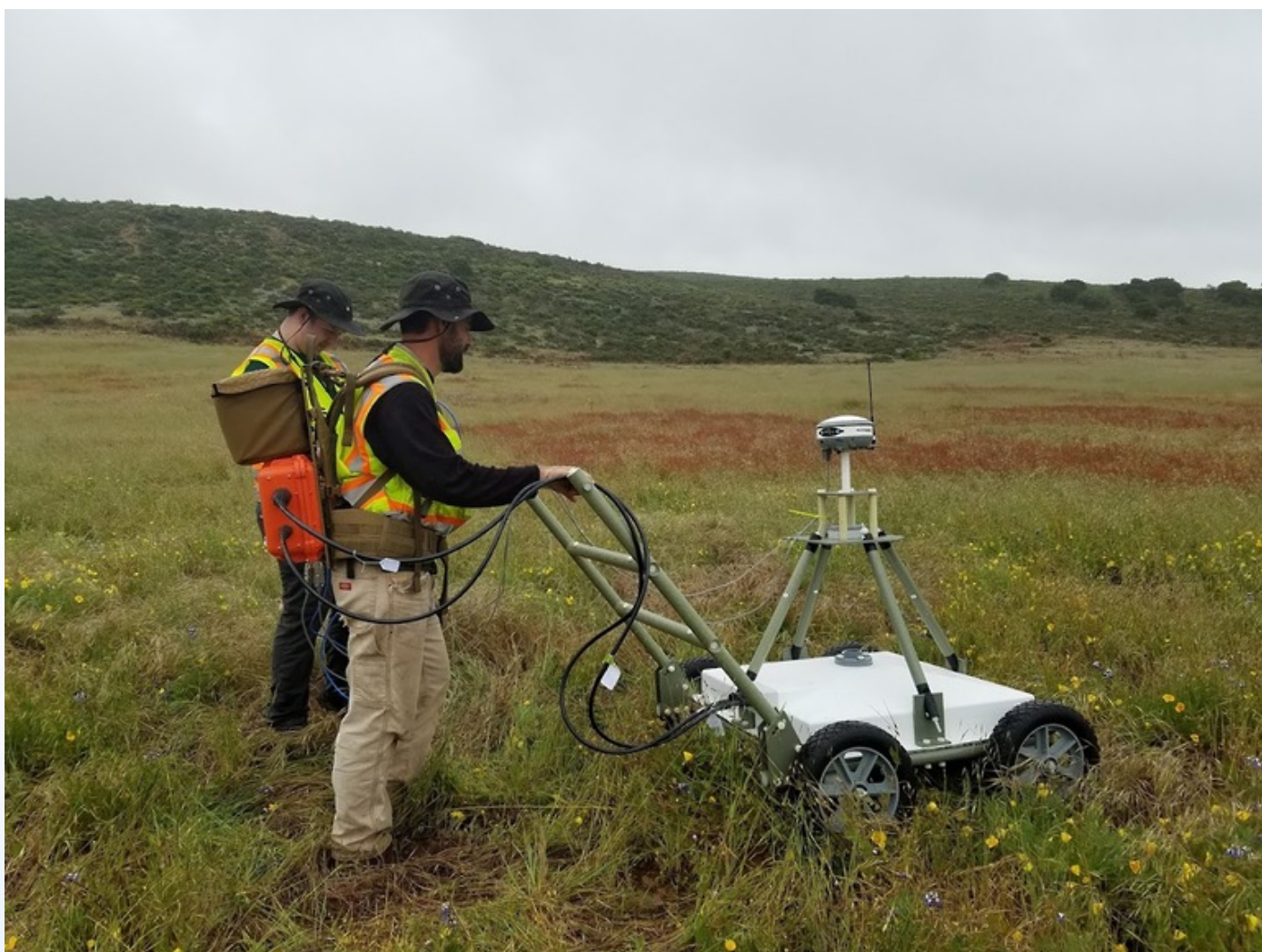
MetalMapper 2x2 being used to locate UXO on a US DoD test range. Image Courtesy of Geometrics Inc.
