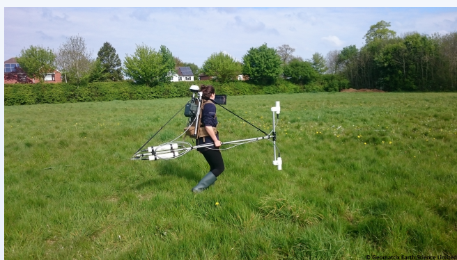
Using MagMonitor in navigation mode to complete a survey
