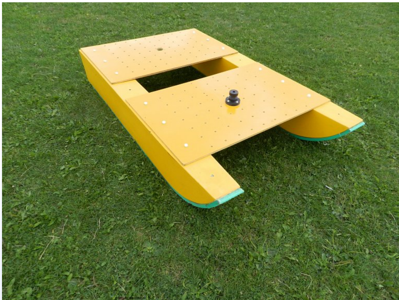
Sledge with tow turret and runners.
