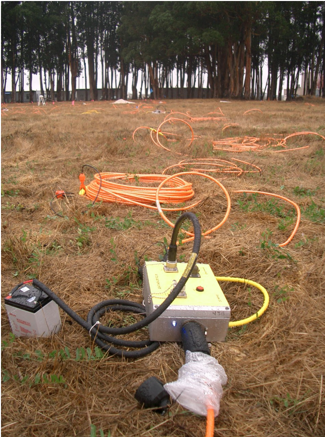
GeodeDZ Seismograph and spread cable
