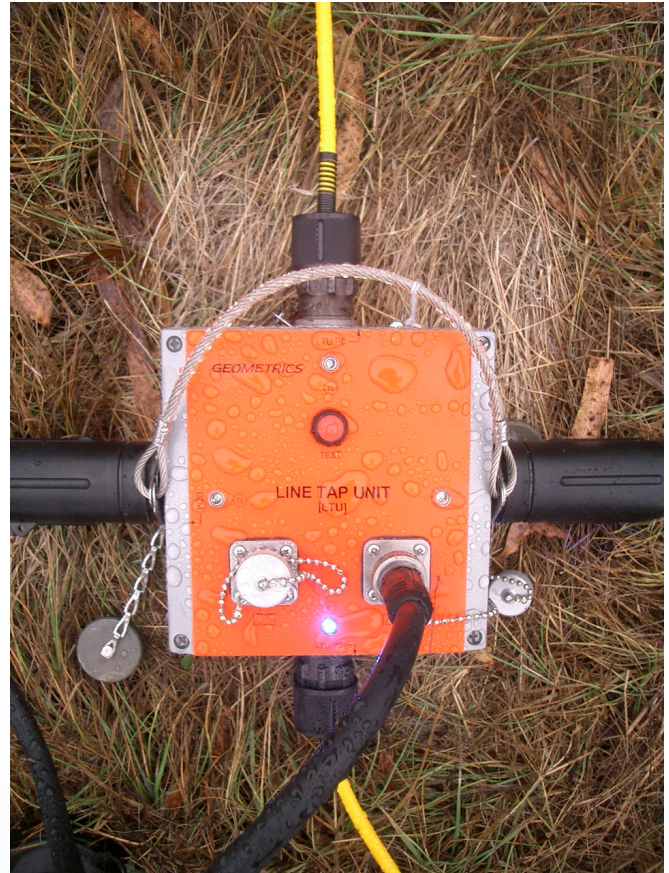
GeodeDZ central line tap unit, used to pass data from each line back to the recording console.
