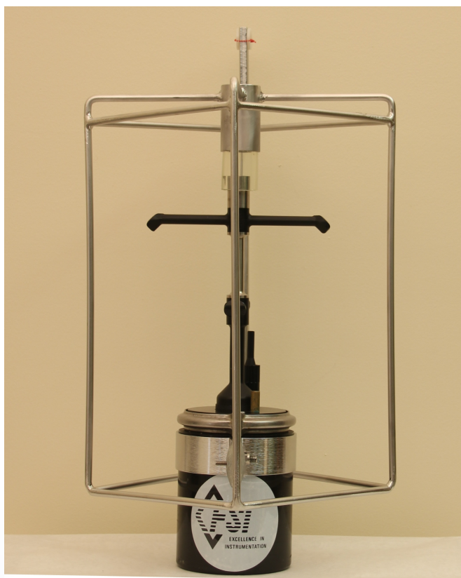
ACM-PLUS with 200m epoxy housing and 1.5 Ton mooring frame.
