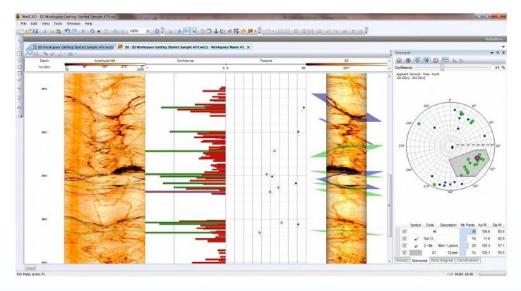
The Image & Structure Interpretation (ISI) module for WellCAD provides a comprehensive tool kit for analysing acoustic logs. Image courtesy of Mount Sopris Instruments.
