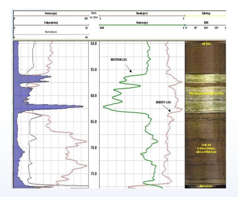
The QL40-NEU Neutron Probe provides users with real-time quantitative porosity measurements in wet, dry, and muddy conditions, enhancing imaging resolution to reveal thin lithological beds. Its advanced design enables precise and reliable data collection in diverse borehole environments, making it an indispensable tool for geophysical investigations.
