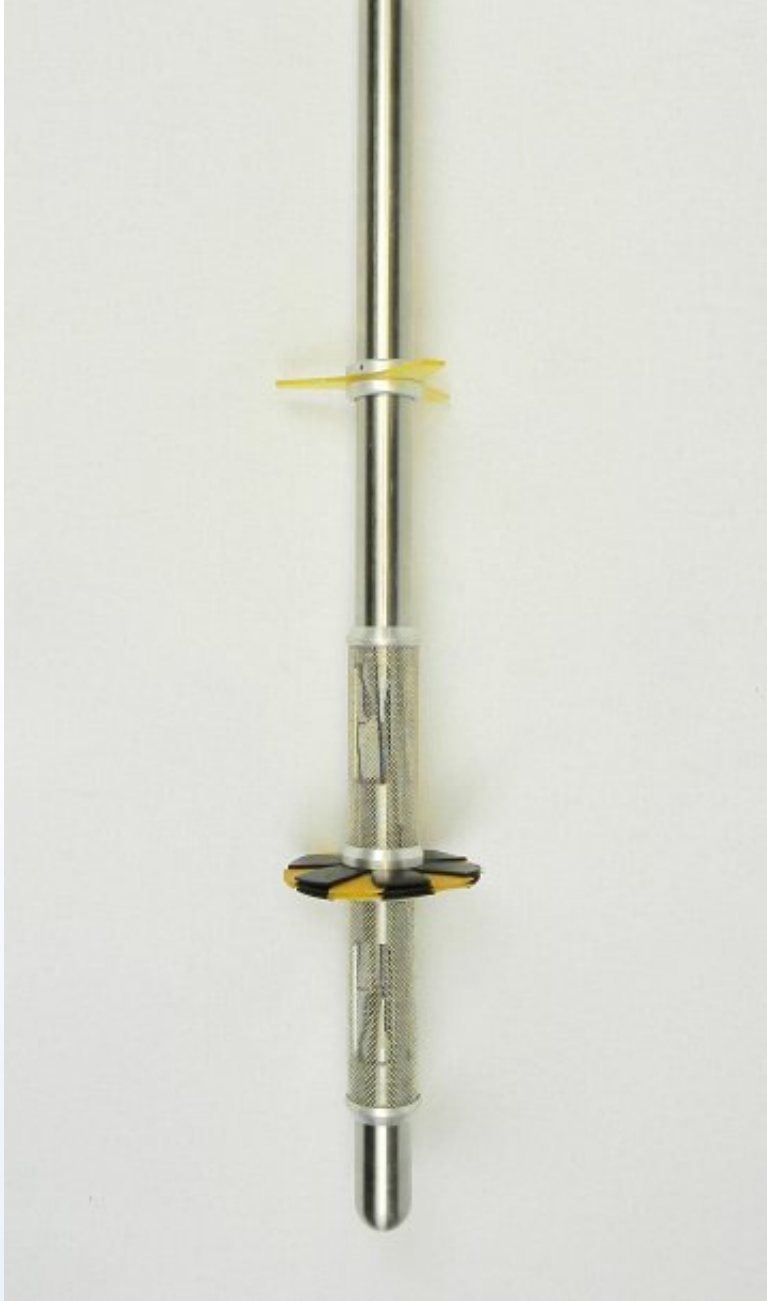
Heat pulse flow meter fitted with centralisers and deviation collar.
