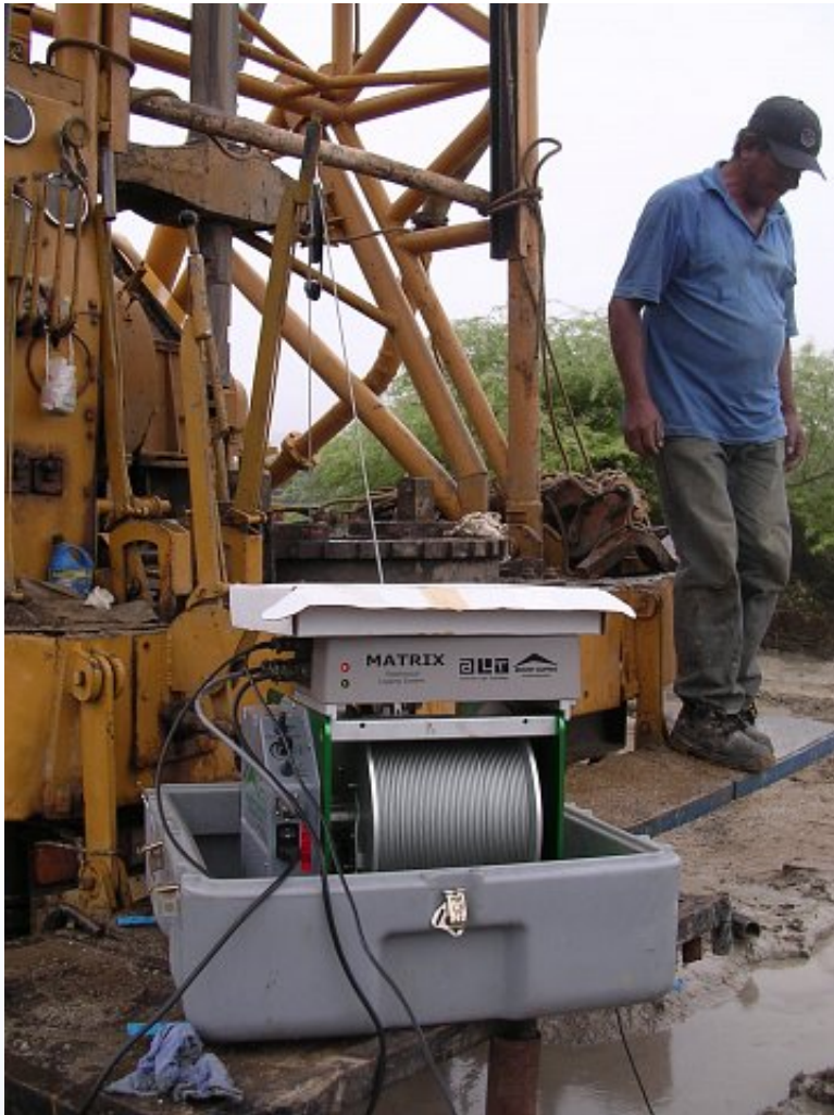
MX Winch deployment off a Drill Rig. Image courtesy of Mount Sopris Instruments.
