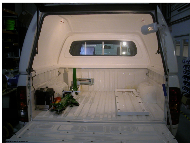
Rear of logging vehicle with integrated winch and probe rack.
