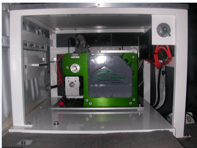
Winch integrated behind the passenger seat of a 4x4 vehicle with inverter for powering the system off the vehicle battery.
