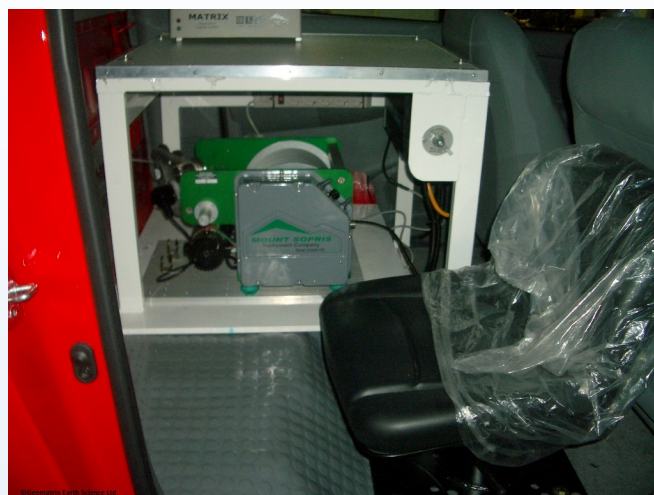
Borehole Logging work station in the back of a Toyota Hilux
