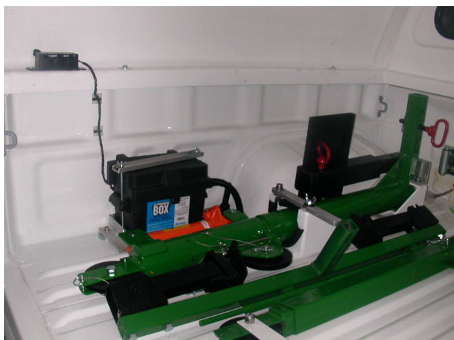
Tow hitch tripod in rear of logging vehicle.
