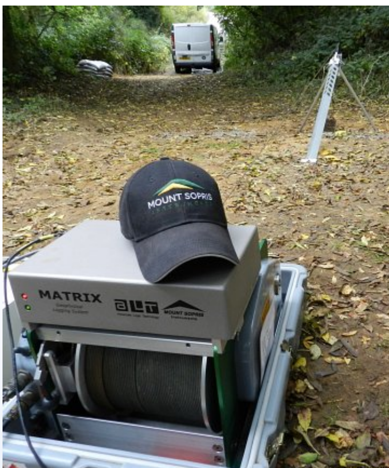
Matrix Logger installed onto MX Winch.
