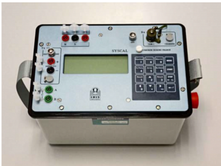
Syscal Junior console (image Courtesy of Iris Instruments)
