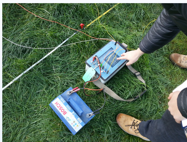
In high resistive lithology with large electrode separations it may be necessary to use an external transmitter battery to support long injection periods.
