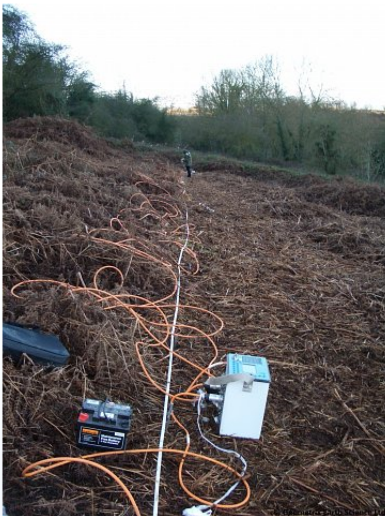
Syscal Pro setup, including external Tx battery.
