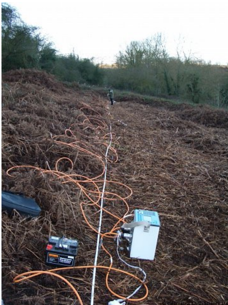
Syscal Pro setup, including external Tx battery.
