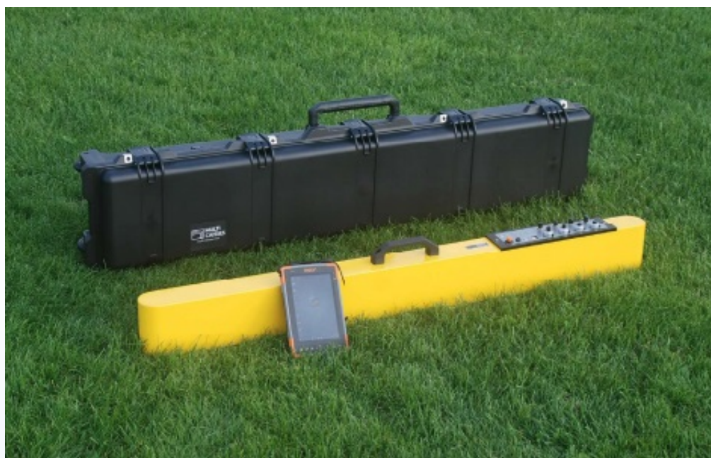
Fig 1. Image of the EM38mk2, including case and an example datalogger you can use with the instrument, Image curteously provided by Geonics Inc
