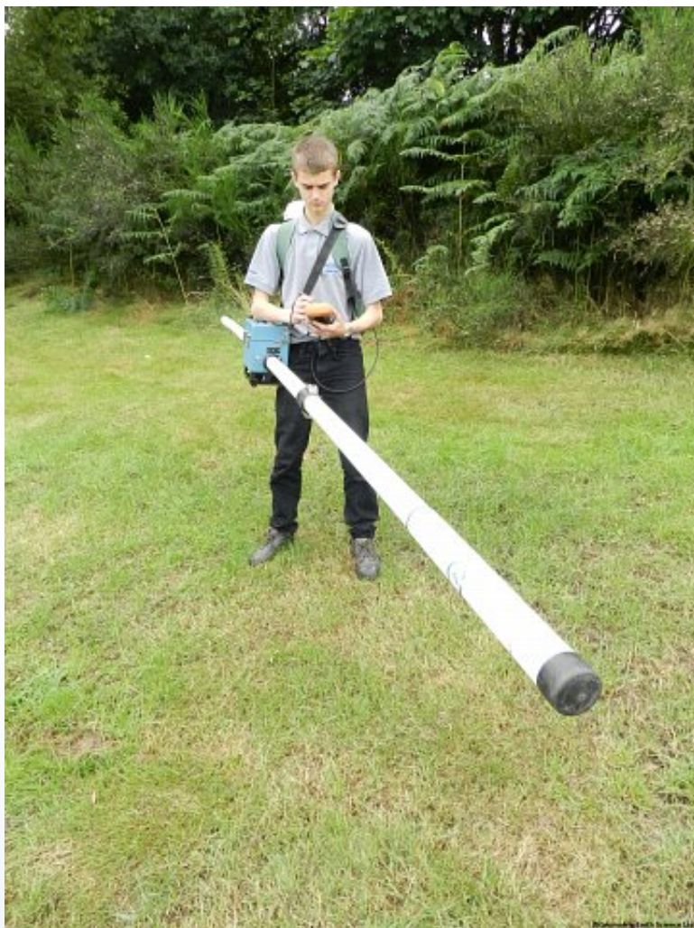
EM31MK2 with integrated GPS.
