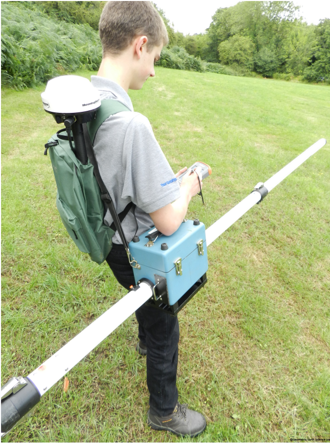
EM31MK2 in operation.
