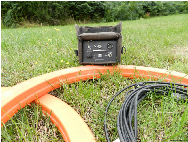
EM34-3 close up of Transmitter
