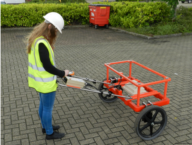
EM61MK2 set-up for typical urban buried tank mitigation survey.
