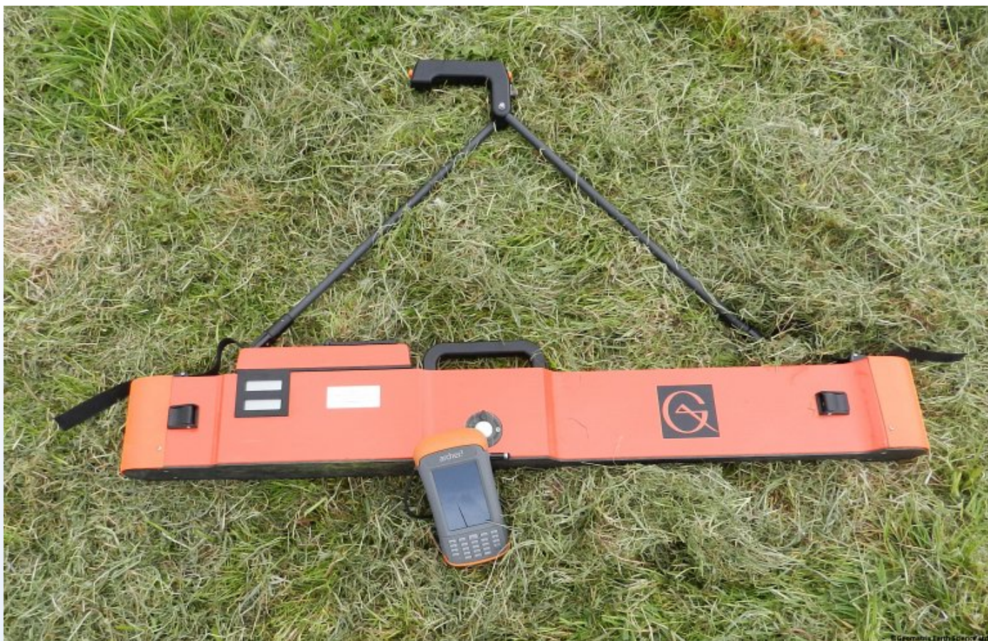
EM38MK2 with ground carry handle.
