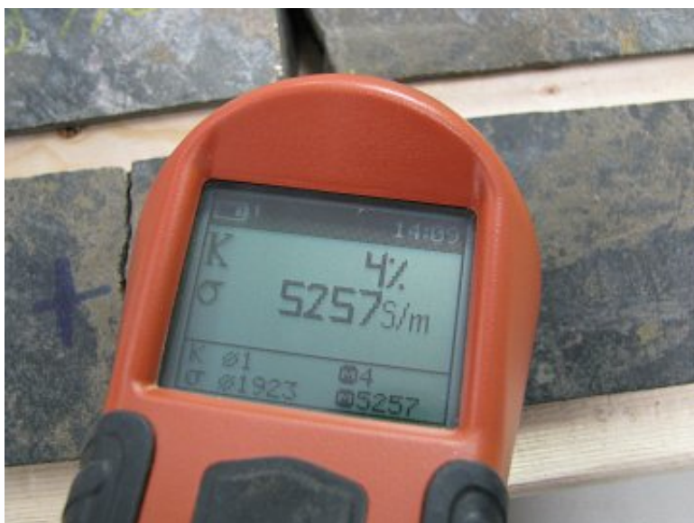
KT10 measuring Conductivity and Magnetic Susceptibility values from a core sample. Image courtesy of Terraplus.
