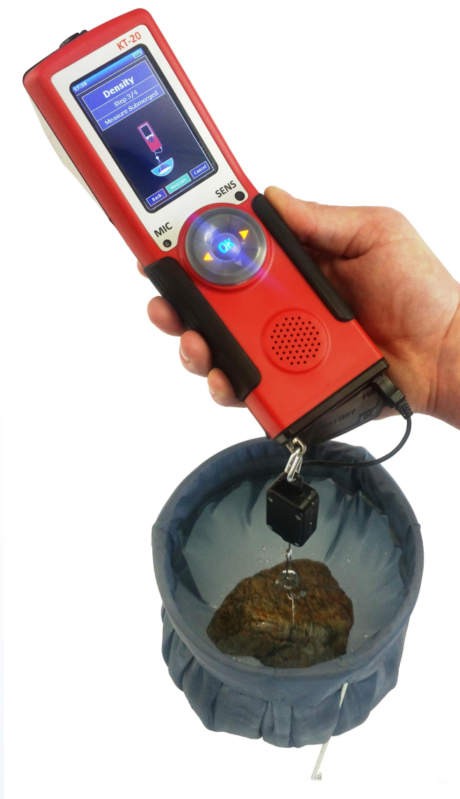
KT20 density measurement- then in water, the density is determined through Archimedes principle. Image courtesy of Terraplus.
