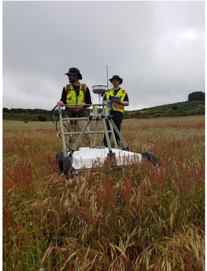
MetalMapper2x2 undertaking a prove-out at Ft. Ord, in Seaside, CA. Ordnance Detection and Discrimination System (ODDS) plot.
