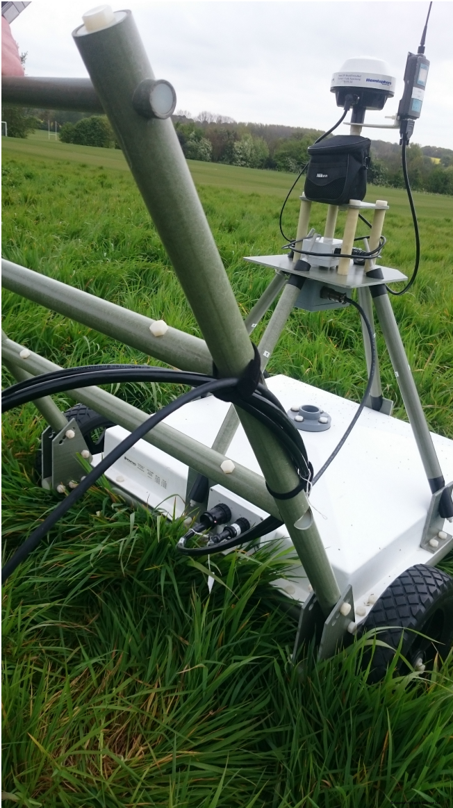
Picture of the MetalMapper2x2 in action at the NSGG test site locating buried mock UXO targets.
