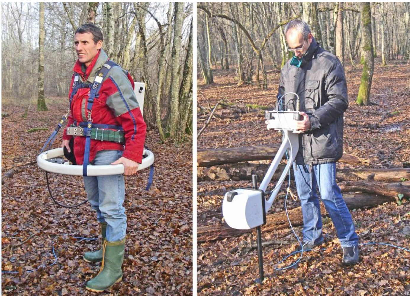
The PROMIS Transmitter coil (left) and 3 component receiver (right) in operation. Image courtesy of Iris Instruments.
