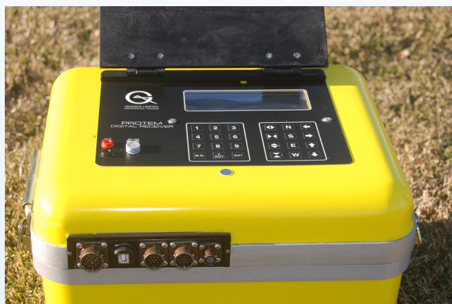
Single channel Transmitter and Receiver TEM system. Image courtesy of Geonics Limited.
