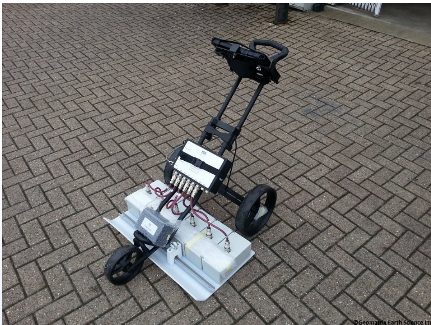
GroundVue 3 8 channel GPR controller configured with 6 1GHz antenna.
