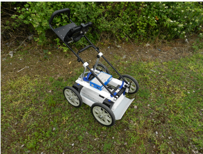
Cart with GV3_8 multi-channel controller and 400MHz GPR antenna
