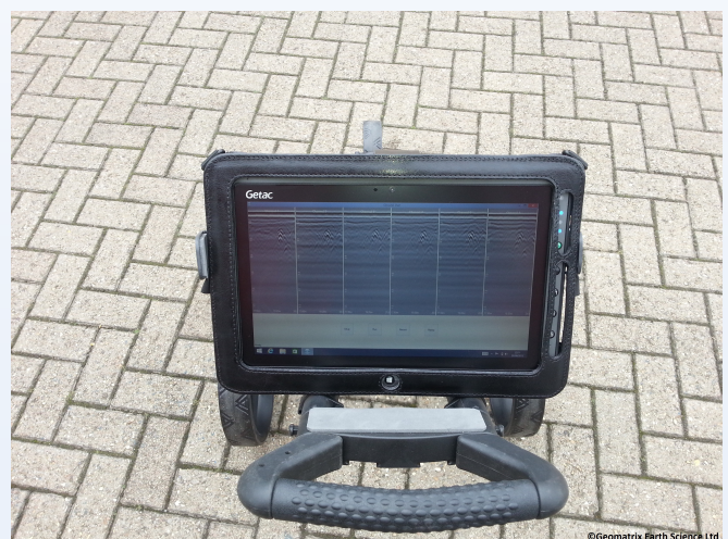
Windows rugged tablet records data via wireless network
