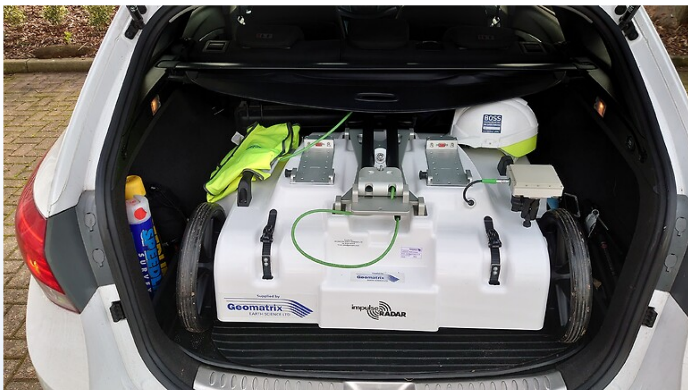
Fig.2 Raptor 45 cart 8ch, packed and transported in an estate car boot
