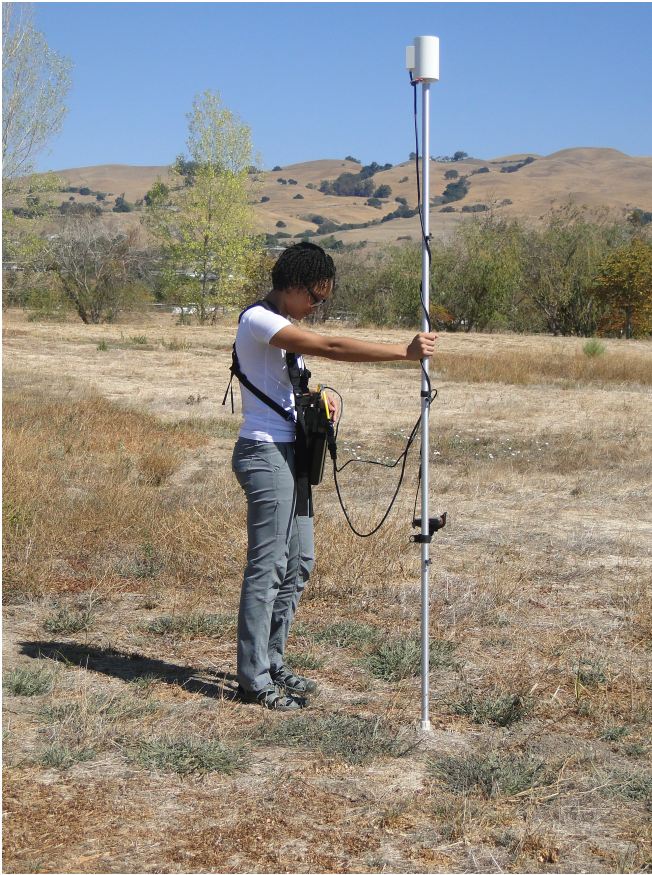
G-857 configured as a roving magnetometer for geological and mineral exploration. Image courtesy of Geometrics Inc
