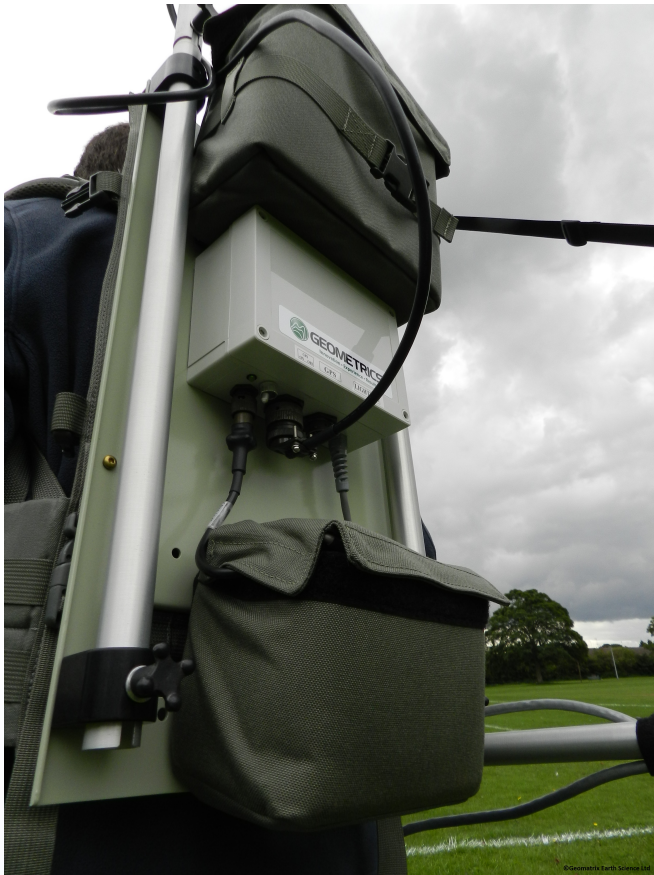
G-858 Backpack, showing battery pouch.
