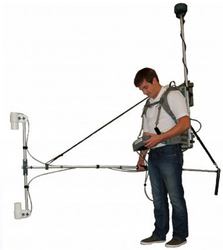
Geometrics G-858 Gradiometer & GPS setup
