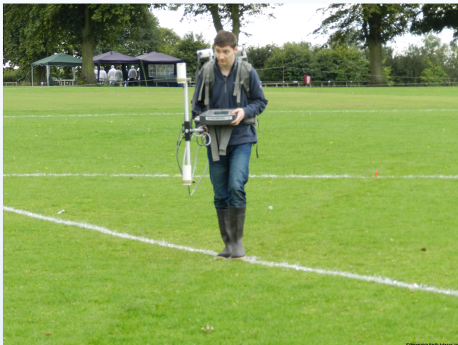
Jonathan undertaking a Heading Error test
