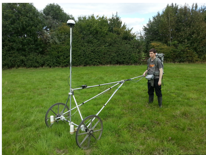
Mag Cart with G-858 gradiometer- sensors are positioned for dual traverse acquisition.
