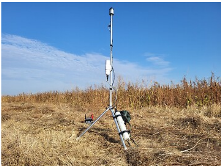
G-862 magnetometer basestation configuration with GPS and data recording module. Image courtesy of Geometrics Inc
