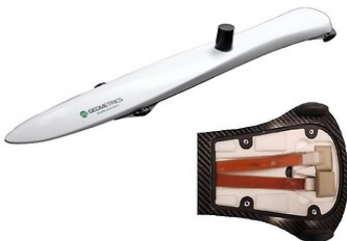
Magarrow II design and the Sensor Orientation
