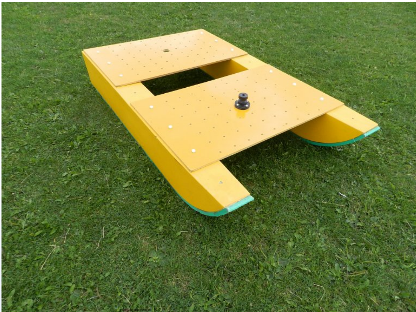
Sledge with tow turret and runners.
