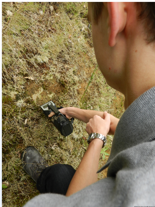
GT-32 measuring natural Gamma count of a rock outcrop.
