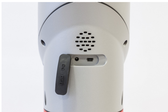
The rear face of the GT40 houses the DC recharging jack and mini USB PC interface connector.
