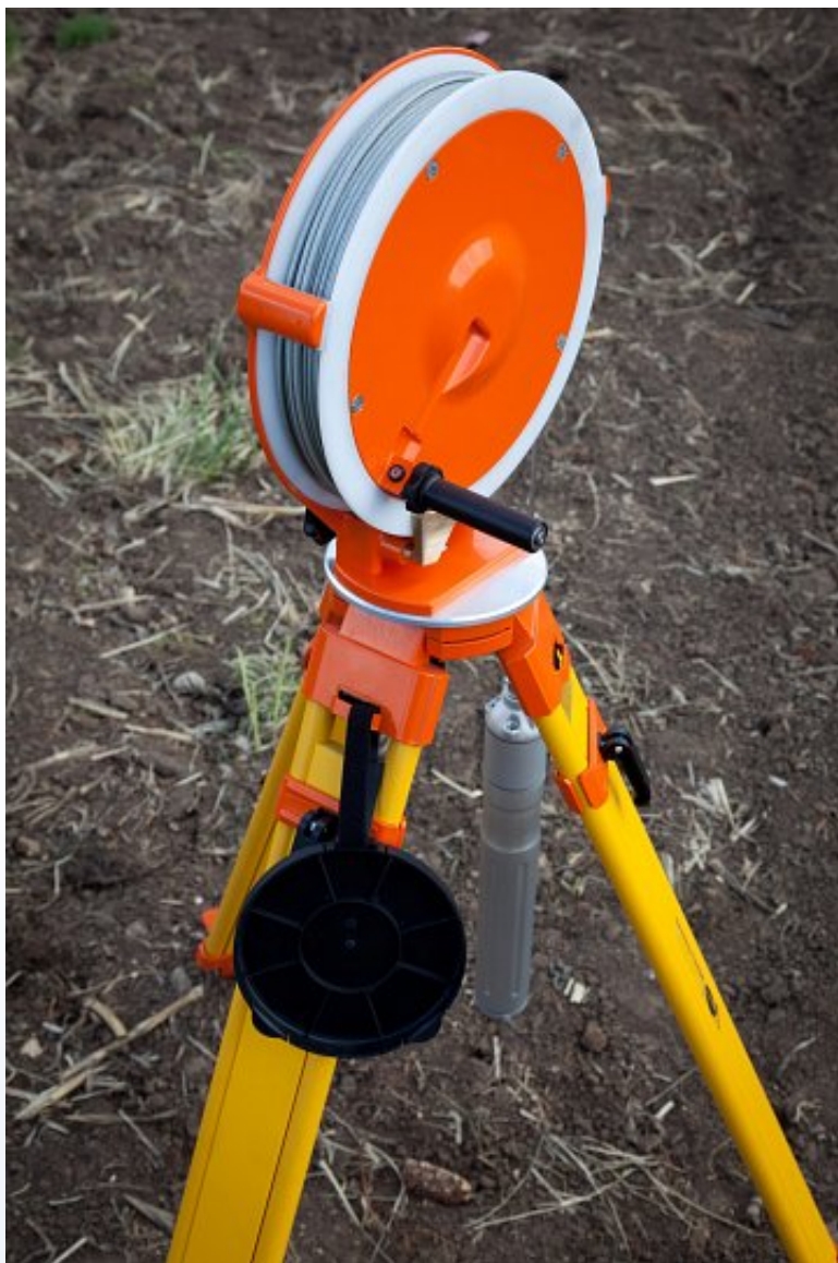
RT-60 borehole gamma ray spectrometer probe. Image courtesy of Georadis.
