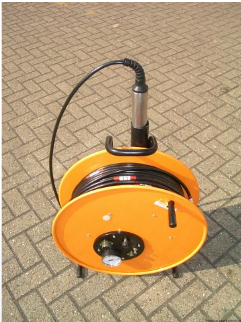
BGK 7 and 100m cable reel.
