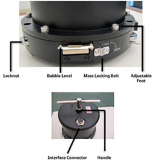
151B features and controls. Image courtesy of RefTek, a Trimble Brand.
