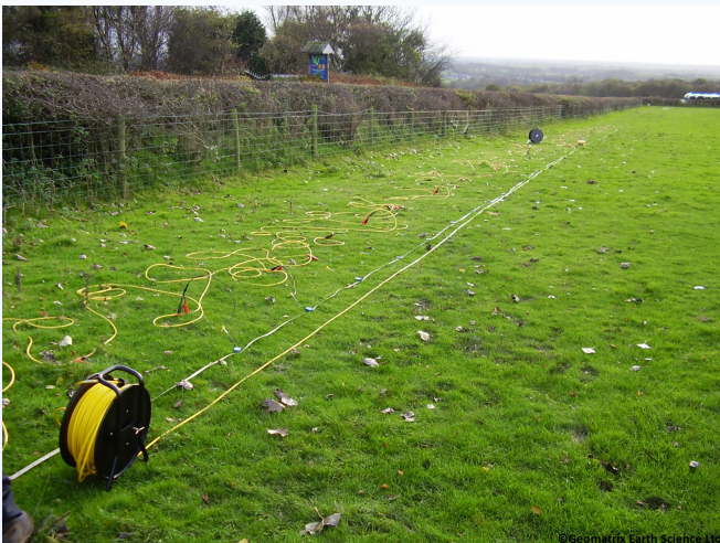
48 channel Geode system for MASW
