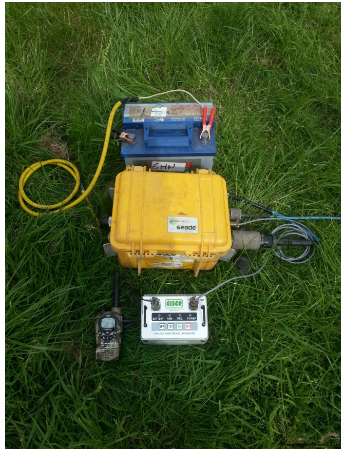
Geode configured with the Gisco radio trigger.
