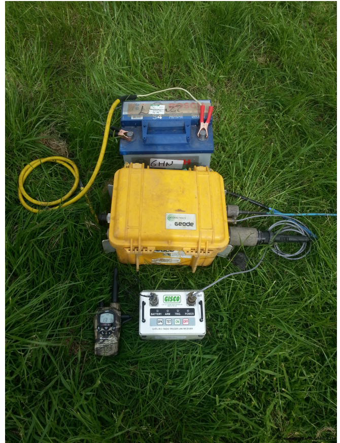
Geode configured with the Gisco radio trigger.
