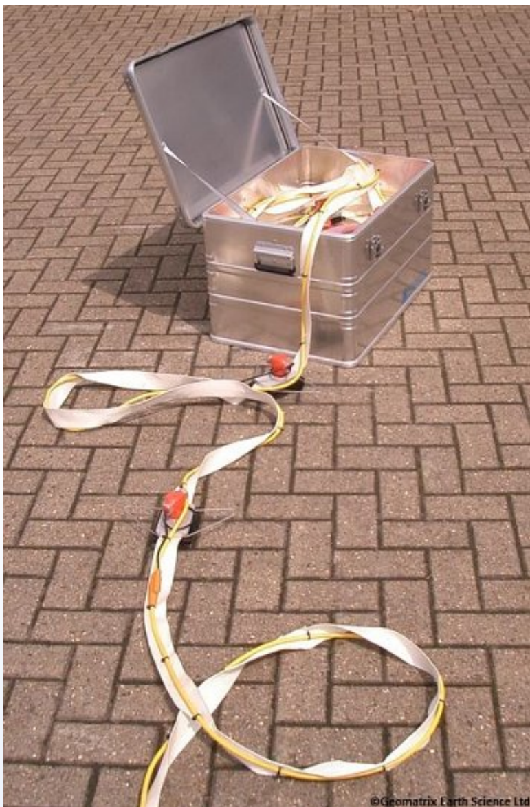
Landstreamer for MASW, 24 4.5Hz geophones at 2m spacings.
