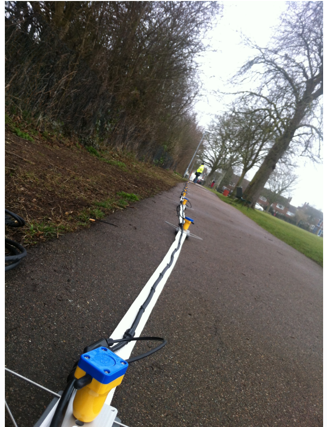
Here is an example of a 48 channel single component landstreamer.
