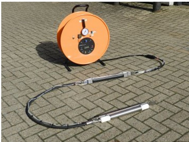
Dual Downhole System (DDS) with two 3 component geophones separated with a 2m interval.
