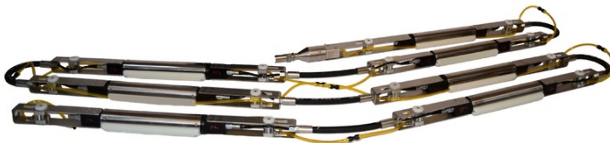
7 station MBAS array with 1m geophone interval. Image courtesy of Geotomographie
