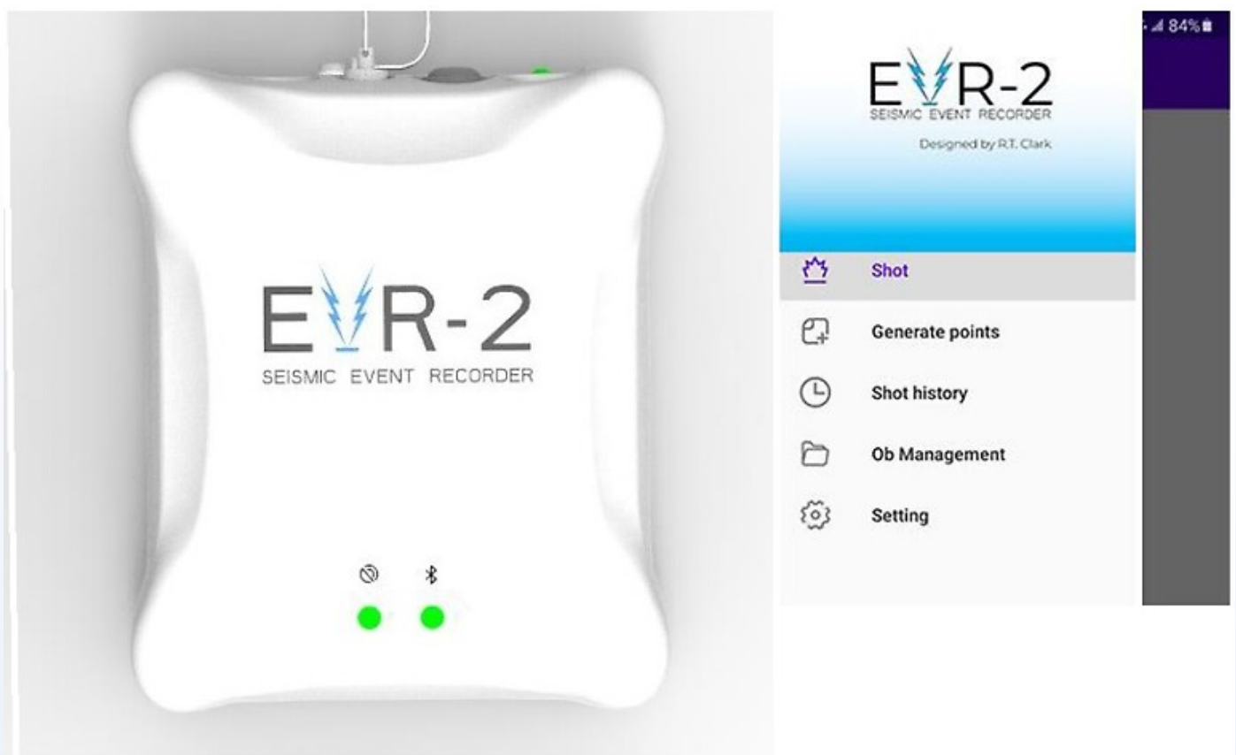
Fig.1. Image of the EVR-2 Seismic Event Recorder unit and on the right is a screenshot of the Android app interface. (Image courteously provided by RT Clark)
