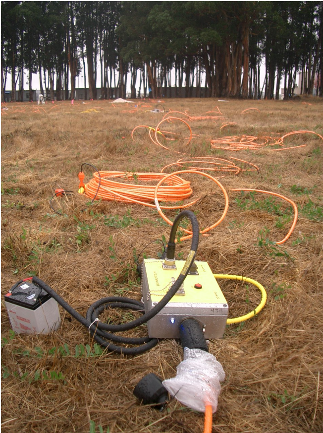
GeodeDZ Seismograph and spread cable
