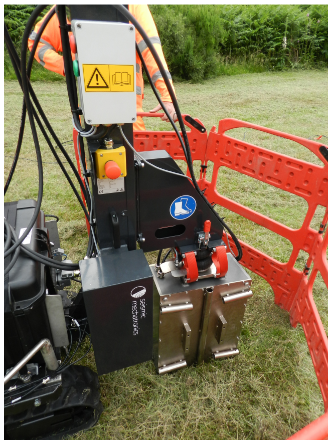
Lightning setup for a P-wave sweep.
