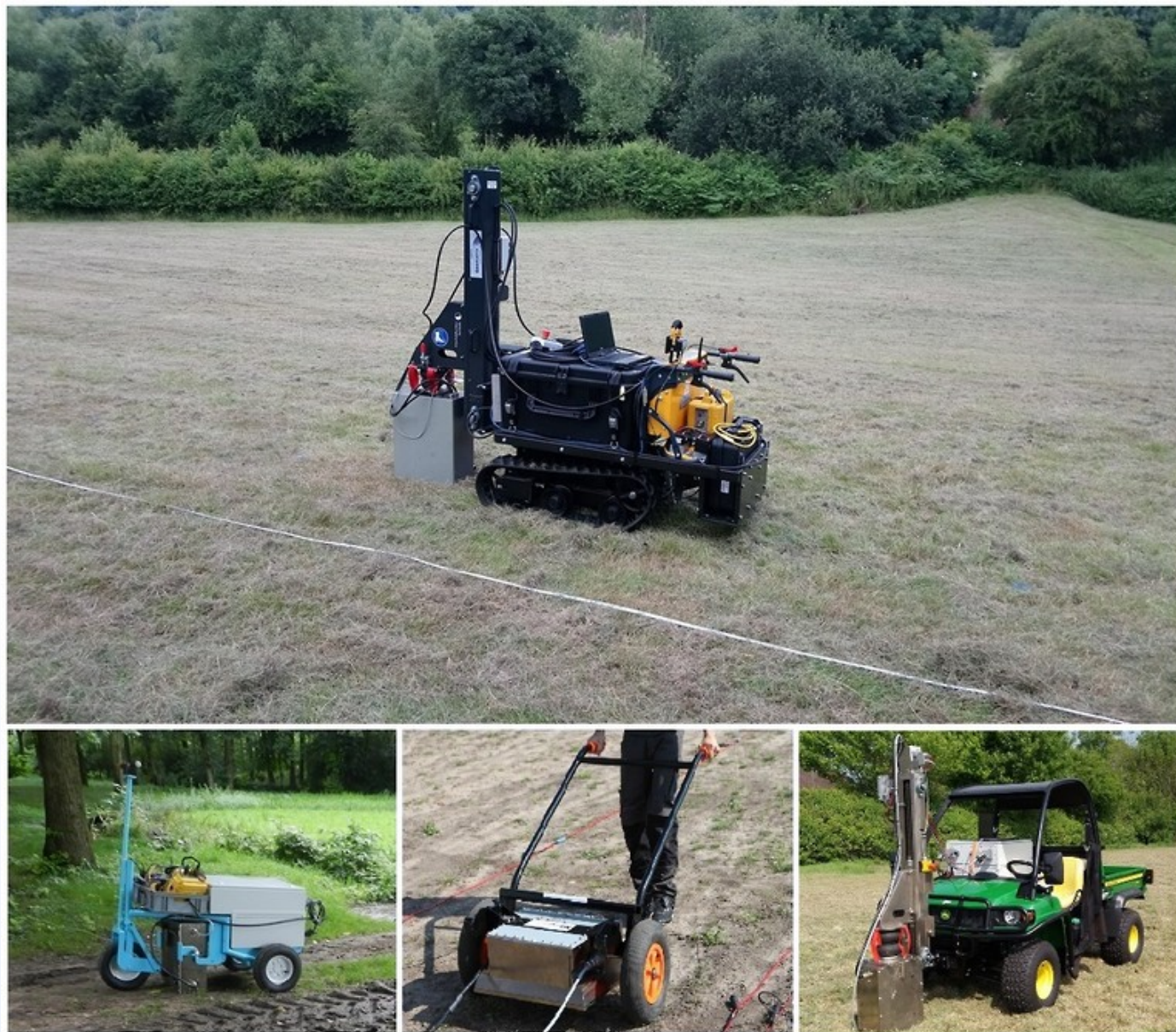
Lightning Seismic Vibrating source mounted to an ATV for deployment on difficult terrain.
