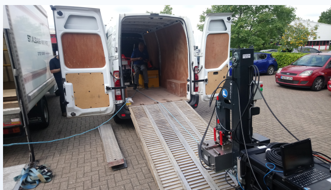
The Lightning can be transported in the back of a high top long wheel based van under a standard drivers licence
