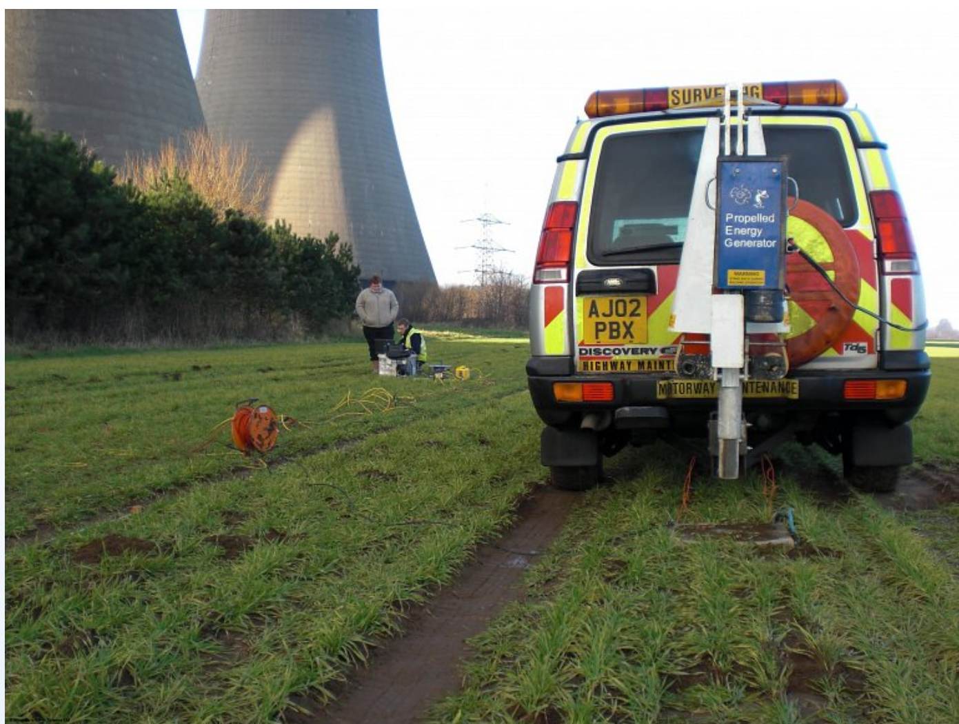
PEG40 seismic source in use alongside a 72 channel refraction spread. Image taken whilst on site with Fugro-GeoServices Ltd.
