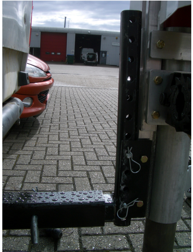
The PEG40 height is fully adjustable to allow the weight acceleration to be optimised for various vehicle.
