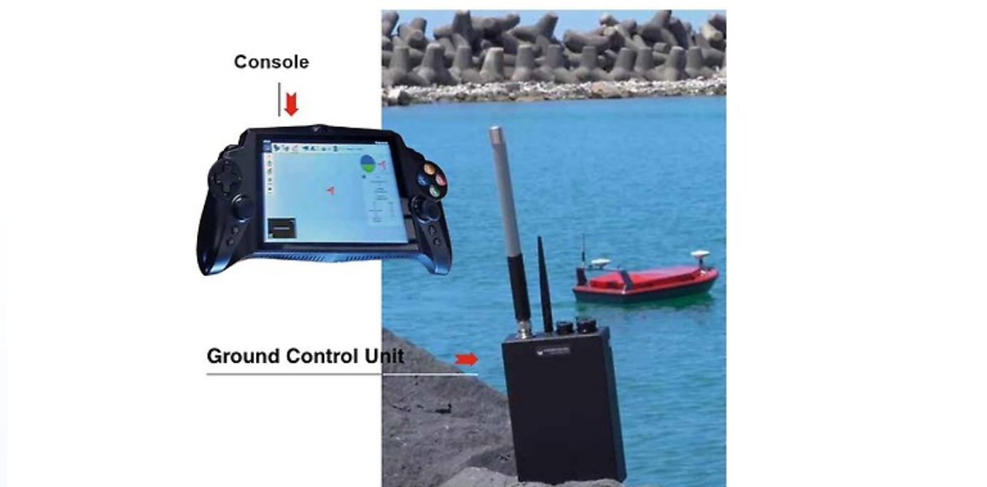
Fig. 3. Sestante autopilot system designed by Codevintec, image shows the ground control unit which fits to the ATV and the smart controller which is used by the operator to control the system, image courteously provided by Codevintec Srl
