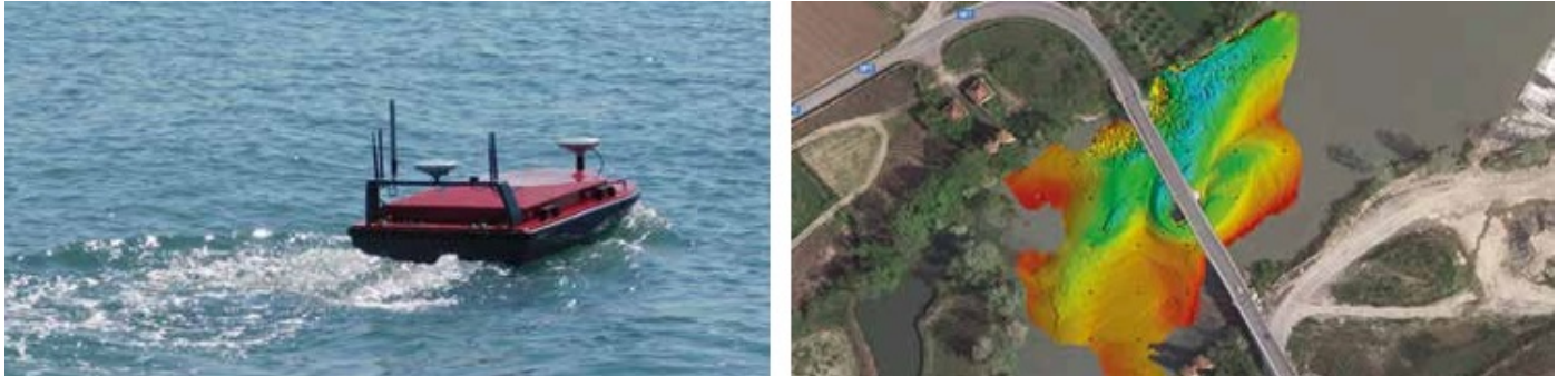
Fig 1. Ck-14 (Made in Italy) with the fitted GPS, antenna and back frame and an example bathymetry dataset captured using the CK14 with sonar. Image courteously provided by Codevintec Srl
