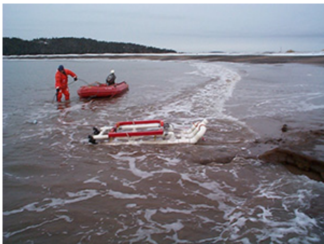
EM61S mounted on PVC sledge for shallow surf zone data acquisition.
