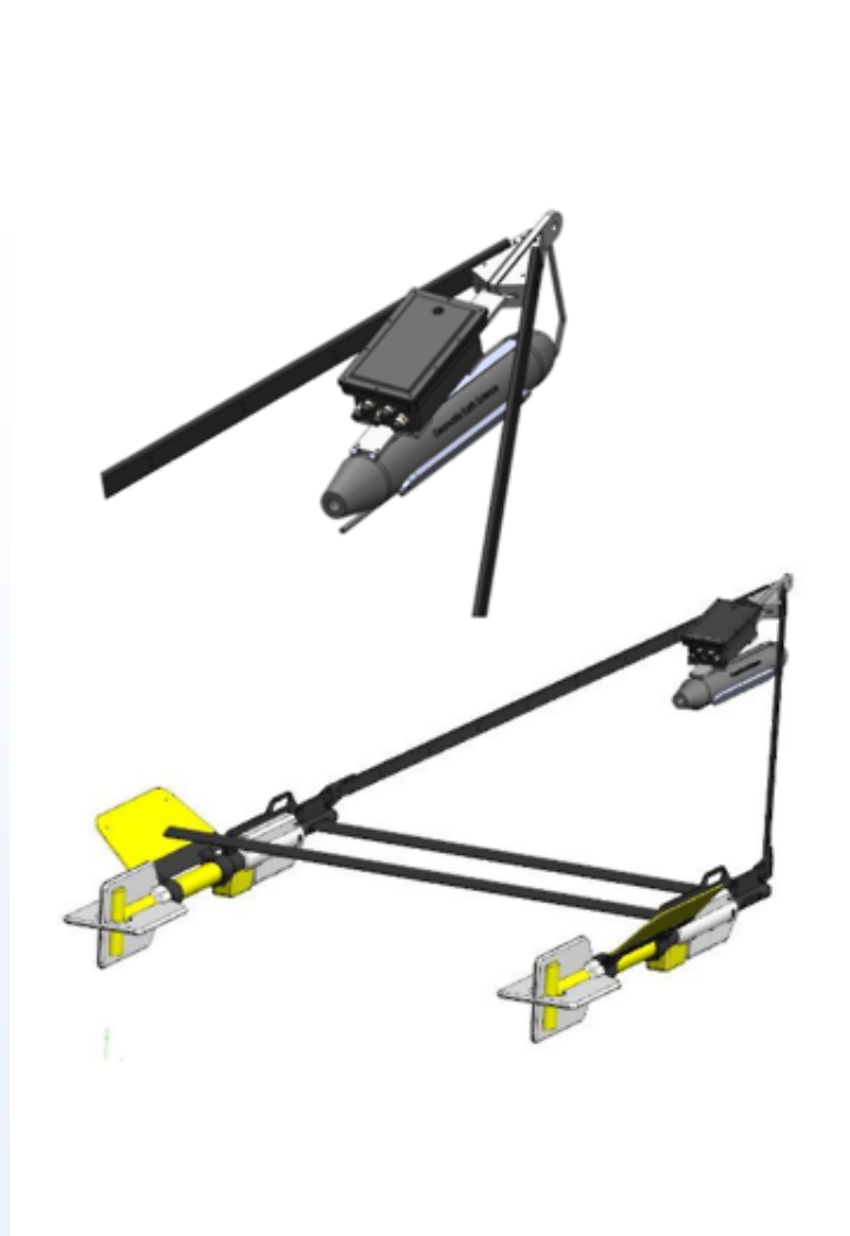
Drawing illustrating the deployment of the QAS? telemetry system on a Transverse Gradiometer Frame with integrated Side Scan Sonar.
