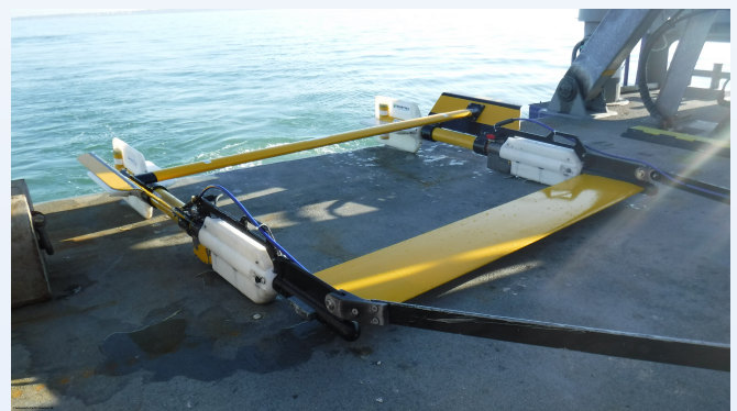
The stream line front spar assembly reduces drag and improving the layback ratio
