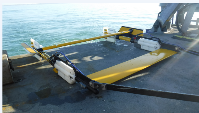
The stream line front spar assembly reduces drag and improving the layback ratio
