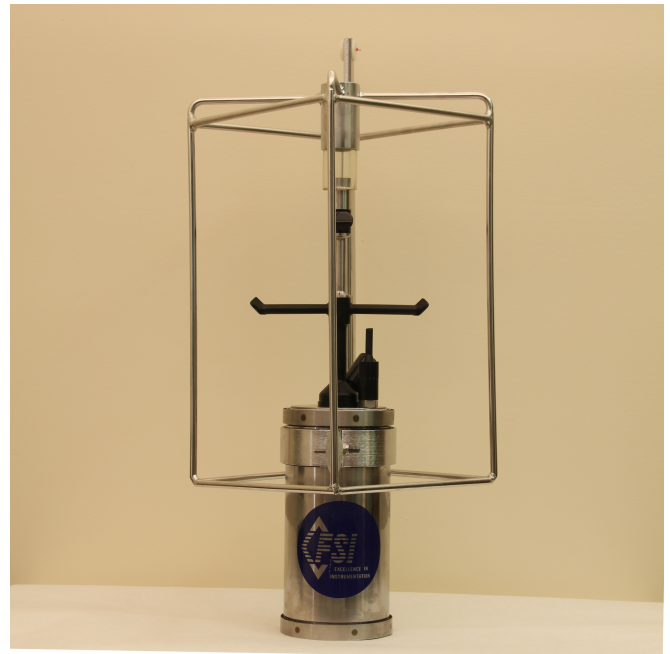
ACM-PLUS with 7000m steel housing and 1.5 Ton mooring frame.
