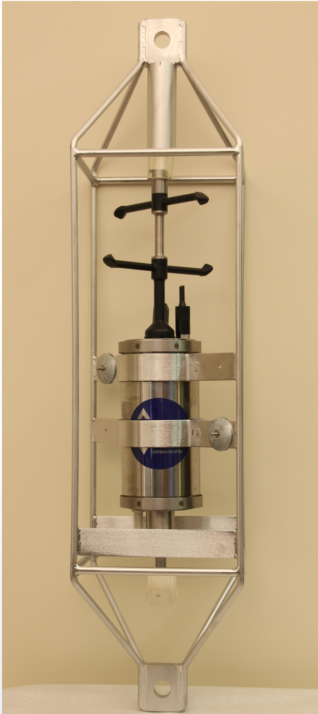
ACM-PLUS with 7000m steel housing and 5 Ton mooring frame and CTD.
