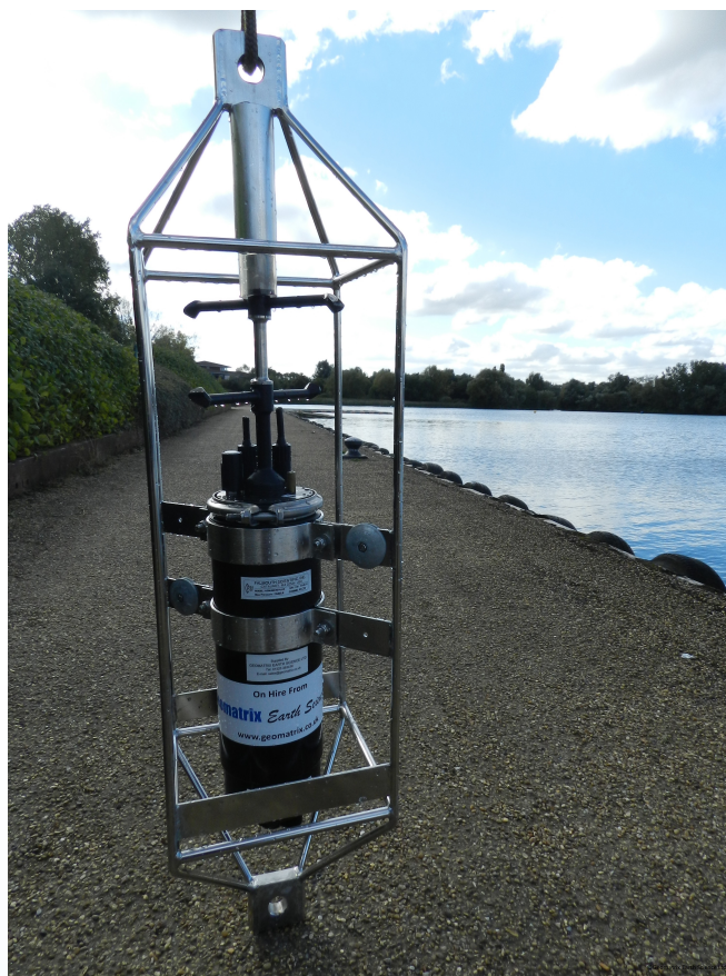
ACM Wave Plus with CTD, auxiliary port and 15 ton frame.
