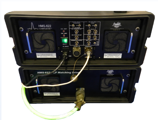
Top end power supply and Analogue A/D electronics module. The secondary module is only required for Low Frequency and Ultra Low Frequency transducers.
